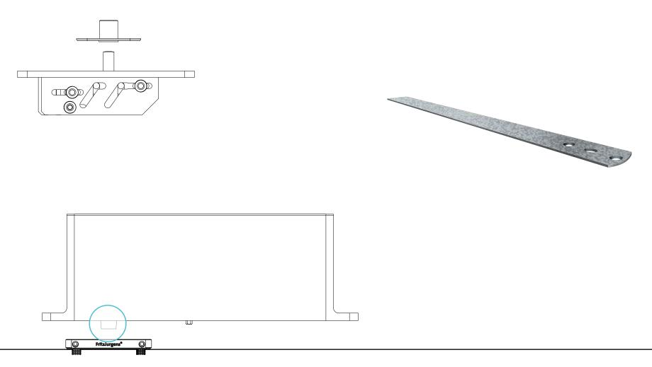
When installing a door fitted with System M, it is very important that the door is installed in its open position. This can be accomplished by using the Axle Wrench to rotate the oval spindle in the bottom of the System M 90°, pointing the arrow toward the direction the door will be opening (0° position). In case of frequent use it is possible to mount the floor plate (art. 400701) on the Axle Wrench.
