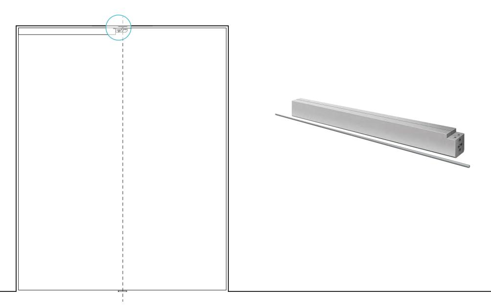
The Hexagon Guide can ease the installation of the pivot door. The minimum distance from the pivot point to the edge of the door is 91 mm and the maximum distance is the middle of the door width. In case the pivot point is more than 280 mm from the edge of the door we offer the Hexagon Guide to ease the installation.
