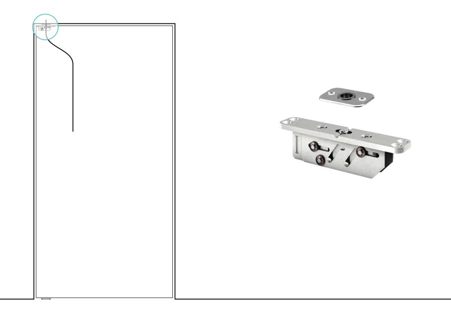
The Cable Grommet is an addition to the existing FritsJurgens top pivot range and enables wiring in the door. This top pivot contains an integrated cable grommet of  $\phi_{7.5}$  mm. This version of the top pivot is available with every FritsJurgens system and replaces the standard delivered top pivot and ceiling plate within a complete set.
